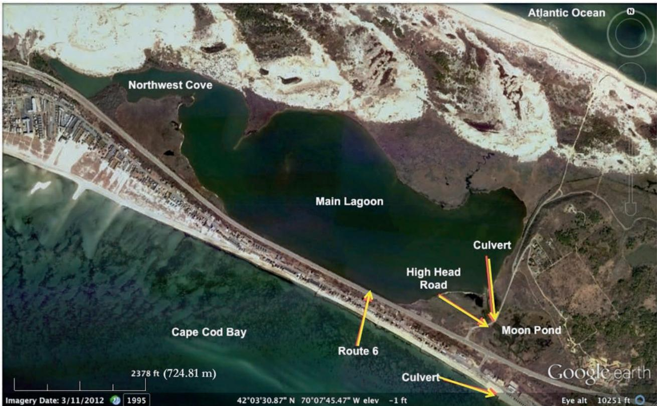
**Figure 1.** Map of East Harbor, Cape Cod National Seashore, MA, depicting three distinct sections: the tide creek (Moon Pond), lagoon, and northwest cove. Culverts are indicated; the 1.22-m diameter clapper valve culvert opened in 2002 is connected directly with Cape Cod Bay, and the culvert under High Head Road is the constriction that limits tidal range in the lagoon. Map Credit: Erica Kidd, Antioch University New England.
